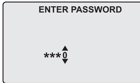
Figure 2.11: Opening the access level
