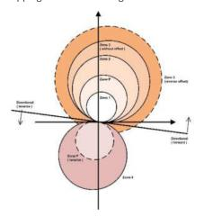
Figure 2: Mho characteristics in P445/P446 (Note - P443 offers additional ZQ)
