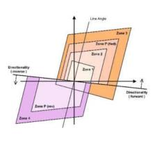
Figure 5: Quadrilateral characteristics in P445/P446 (Note - P443 offers additional ZQ)
