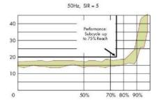
Figure 3: P443/446 sample min-max timing contour: 50 Hz, SIR=5
