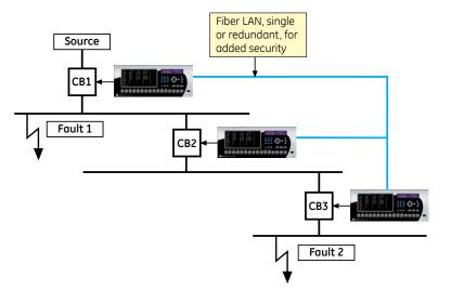
Reverse zone interlocking protection. By using the IEC 61850/GOOSE or hi-speed direct I/O capability blocking signals can be transferred upstream, allowing for minimal coordination delays. Fast clearance can be provided for Fault 1 while still maintaining coordination for Fault 2.
