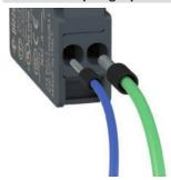
The PUSH-IN spring connection allows quick and simple wiring, as the wire just needs to be inserted into the appropriate hole in order t establish the electrical connection and automatically secure the wire The reduced force required to insert the wire allows completely tool-free connection by using wires with crimped wire-end sleeves. They are released by pressing a special wire release button - including individually - with any tool, without the need to use a screwdriver of a predefined size.
