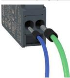
The PUSH-IN spring connection allows quick and simple wiring, as the wire just needs to be inserted into the appropriate hole in order t establish the electrical connection and automatically secure the wire. The reduced force required to insert the wire allows completely toolfree connection by using wires with crimped wire-end sleeves. They are released by pressing a special wire release button - including individually - with any tool, without the need to use a screwdriver of a predefined size.
